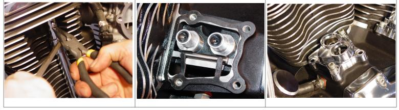
The hight of the lifters and length of 6. the Pushrods make it tricky to install without removal of the rocker covers and breather/rocker arm supports. The Pushrods may be installed if inserted into the heads as an assembly with the Pushrod tubes and lifter blocks.
