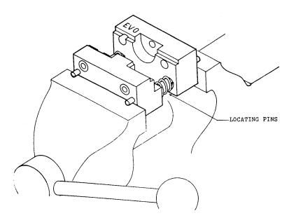
Tappet Roller Tool Must be Mounted in a Common Bench Vise as illustration shows. Springs must also be mounted on locating pins when tool is in use. This is the only way this unit can correctly be used. If used in any other way locating pins may break.
