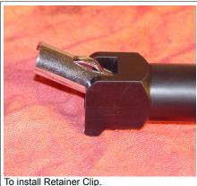
Place the retainer Clip into the tool as shown.
