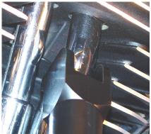
2. Slip the retainer Clip into the top grove and place the tool on top of the spring cover as shown. Pivot the tool upward.
