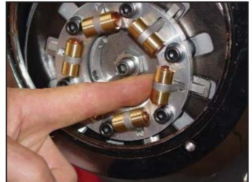
6. Check the movement of each weighted arm for freedom of movement. Insure the arms are riding on the spider fingers.
