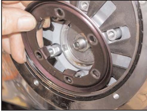
2. The spring plate is now free to be removed from the clutch.
