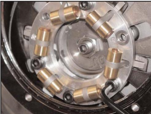
5. Install the VPC onto the pressure plate using the six metric Allen cap screws and washers supplied in the kit.
