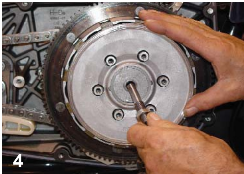
4. A & B - Remove the OEM jam nut and clutch adjuster from the stock pressure plate. They will be re used. Remove the OEM pressure plate.
