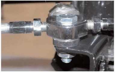
6. Using Loctite, secure the brake block on to the frame insuring sufficient room for the brake line wires. A spacer may be necessary.
