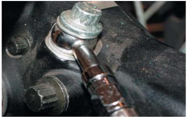
1. The master cylinder does not have a flare in the outlet port. 2. Working from the rear caliper we installed a banjo fitting (VT You will need a banjo fitting and bolt or a flare fitting to install No. 23-4047) and a 12 "Russell brake line (VT No. 23-8020). the front section brake line. On our installation we selected the proper fitting (VT No. 23-1988) and 150 degree line (VT No. 23-4284).
