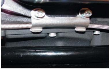
7. Secure the brake line as shown.
