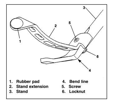
7. Place stand in its extended position. Carefully remove support blocking from beneath motorcycle frame.
