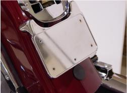
10. Select the desired turn signal lamps and mount as necessary. V- Twin offers a wide selection of custom lights for this application.
