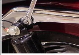
5. Remove the four hex head screws and internal- tooth lock washers to release the license plate bottom support tube from the rear frame rails.
