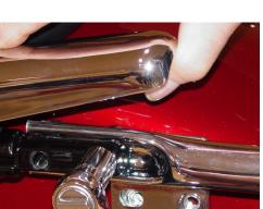
6. Install the new eliminator brackets with nuts supplied in kit onto the frame using light lens and the OEM turn signals. A the hex head screws and lock washers new stop light lens(VT # 33-0256) is removed in step 5. Fasten the saddlebag required to insure the new license plate support bracket using the T-40 TORX screws removed in step 2 and nuts suppled in kit. Tighten the screws to 15-20 ft-lbs.
