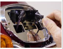
8. Unplug the OEM turn signal lights 9. Using the OEM bolts attach the new
