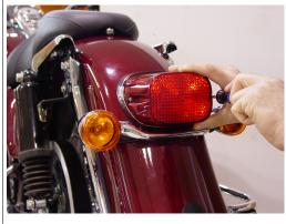
and remove the 2 bolts securing the license plate. signal assembly. Retain the bolts.
