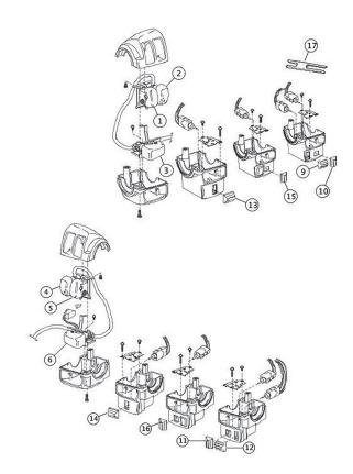
Figure 5. Service Parts: Chrome Handlebar Switch Caps Table 2. Service Parts: Chrome Handlebar Switch Caps
