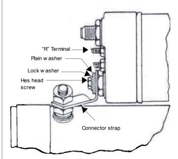
For field coil connection use short hex head screw, lock washer and plain washer. If old unit did not have "R" terminal disregard.
