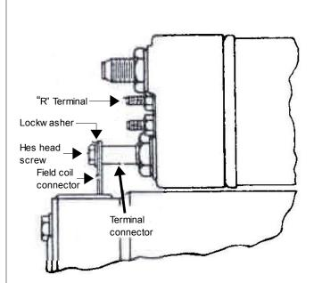
washer & copper tube as per illustration. If old unit did not have "R" terminal, disregard.
