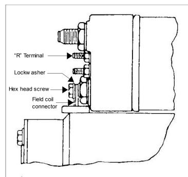
For the field coil connection use short hex head screw and For field coil connection use long hex head screw, lock lock washer. If old unit did not have "R" terminal, disregard.
