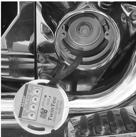
3. You can completely remove the OE ignition harness and external module (1980 and later models) if desired. However, you must disconnect all OE wires from the coil except the white/black wire from the engine stop/run switch.
