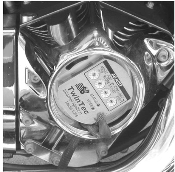
Figure 3A - Finished Big-Twin® Installation
