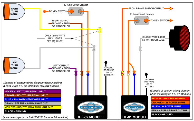
The wire colors in the drawing are used for reference only based on the colors we use on our module. When installing either the IHL-01 or IHL-02 3 HI/LOW Intensifier Modules on a factory model, be sure to consult your bikes service manual for exact wiring diagrams and color descriptions to achieve proper installation.
