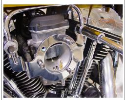
7. Apply light grease to the gasket and place on the air filter baseplate. Mount the Filter and baseplate using the 1/4-20 X5/8 screws. Torque to 3-5 Ft. Lbs.
