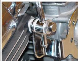
5. Slide a gasket between the support bracket and 6. Torque the Banjo bolts to 10-12 Ft. Lbs. the carburetor/EFI unit. Light grease and the 1/4 -20 bolts can be used to hold the gasket in place
