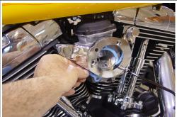
4. Slide a gasket between the support bracket and the carburetor. Light grease and the  $\frac{1}{4}$  -20 bolts can be used to hold the gasket in place
