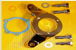
2. The kit is supplied with 3/8 and ½ inch Banjo bolts. Install the spacers as needed.
