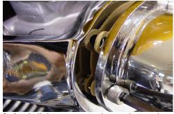
6. Apply light grease to the gasket and place on the air filter baseplate. Mount the Filter and baseplate using the supplied hardware. Torque to 3-5 Ft. Lbs.
