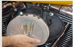
1. Using the Service Manual Remove the OEM Air Filter assembly.
