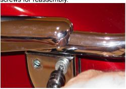
securing the saddlebag support bracket the front saddlebag mounting bracket to
