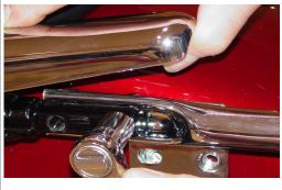
6. Install the new luggage rack onto the 7. Fasten the saddlebag support bracket screws to 15-20 ft-lbs.
