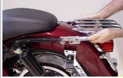
frame using the hex head screws and lock using the T-40 TORX screws removed in washers removed in step 5. Tighten the step 2. Tighten the screws to 15-20 ft-lbs.
