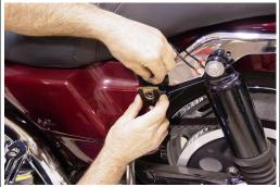
chrome frame cover. Remove the cover. Retain the hardware for reassembly.
