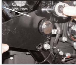
Place the supplied plate, washer and bolt as shown and start the bolt most of the way in.
