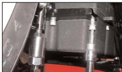
6. Install the bracket using the new bolts and washers. Torque to 10 ft-lbs.
