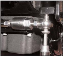
7. Adjust the length of the strut to allow proper alignment and install the provided 3/8 button head bolt. The strut has a left and right hand thread to allow adjustment of equal length.
