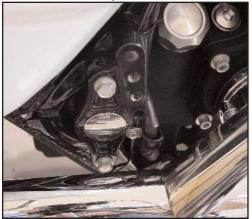
1. On motorcycles with OEM exhaust the right side exhaust pipes must be removed to access and remove the lower bolt on the swing arm side plate. Check to see if you need to loosen or remove the right side exhaust on your bike. If necessary accomplish this first.
