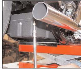
5. Remove the 3 rear socket head bolts from transmission rear oil pan.
