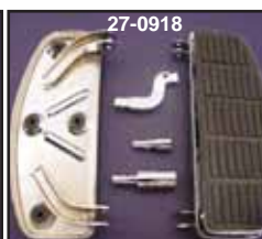
Chrome 'D' Shaped Footboards include rubber pads. The 1974-up Iso boards feature a raised footboard pad with anti-vibration rubbers. Sold in pairs.
