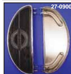
Oval Style Shape Footboards fit the stock mounting brackets on 1940-84 FL. Footboards replaces 50603-40.
