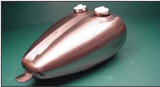
3.3 Gallon Axed Cap features dual cap design and universal mount tabs. Use 3/8" NPT petcock.
