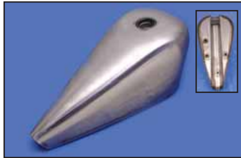
Mini Sporty Tank features bottom mount design with 2.5 gallon capacity and bung style filler neck. VT No. 38-0476
