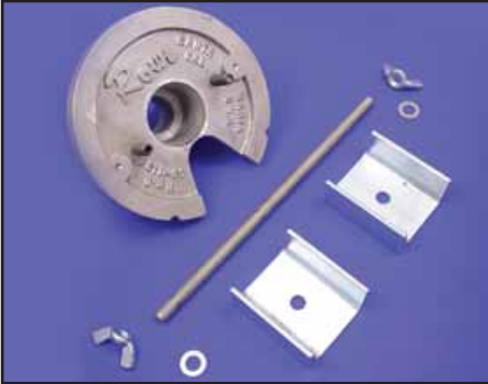
Flywheel Rebuilding Fixture. Allows servicing and disassembly of flywheels in a standard shop vise. Holds unit from turning when tightening nuts, when installing or removing sprocket and pinion shafts. VT No. 16-1002
