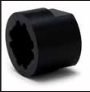
Flywheel Rebuilding Fixture. Allows servicing and disassembly of flywheels in a standard shop vise. Holds unit from turning when tightening nuts, when installing or removing sprocket and pinion shafts. VT No. 16-1002
