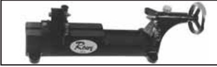
Original Style Factory Type Crank Truing Machine features cast Iron Construction. Designed to true stock style fly wheels. 10" swing right side, 6" swing left side, 18" maximum center to center. Weighs over 80 pounds. VT No. 16-1000
