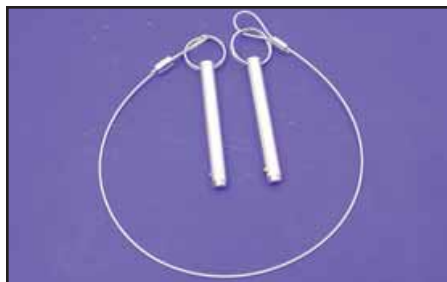
Balancer Shaft Retention Pin use this tool to secure the engine balancers on TC-88B engines when servicing flywheel assembly. This tool locks into the balancers sprocket pin holes to prevent the balancer from turning out of sync with flywheel. VT No. 16-1163
