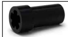
Balancer Shaft Removal Tool designed to remove both front and rear counter-balancer shaft bearing assembly, from the left engine case on the new 96" and 110" Beta engines. VT No. 16-1374
