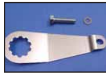
Crankshaft Stabilizer Bracket acts as third hand. Sliding over crank splines, and bolting to a primary mount hole prevents crank from turning while installing pistons, cylinders or rings. VT No 16-5051
