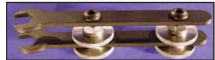
Sifton Pushrod Adjusting Wrench eliminates the need for 3 hands, dual wrench holds 2 outer nuts. The inner is tightened with a separate wrench, fits 7/16" hex nuts and is fully adjustable for solid lifters. VT No. 16-0819
