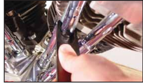
Sifton Pushrod Adjustment Gauge for use on Big Twins 1953-84 with hydraulic lifter. Replaces 91438-79. Complete with instructions. VT No. 16-0993
