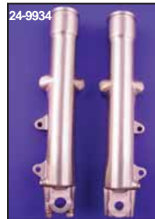
1980-83 FXWG Lower Legs feature smooth design without reflector boss, for dual disc 10" applications. Internals not included, replaces 45872-80 and 45871-80.
