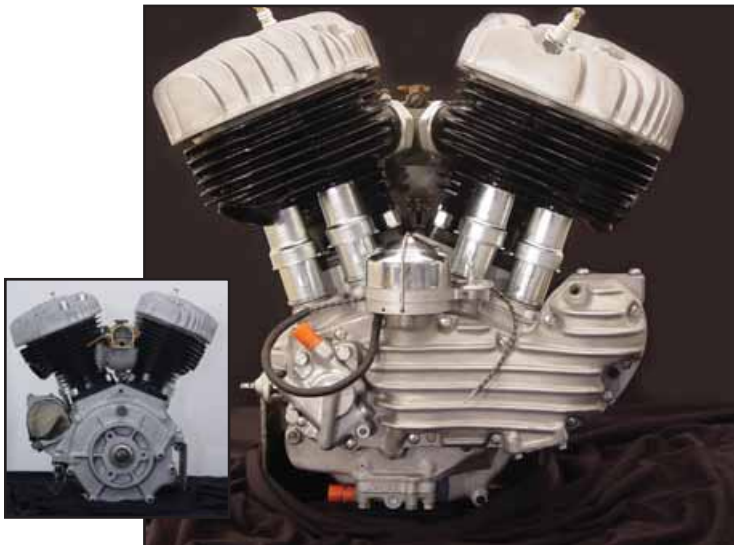
80" ULH Flathead Rebuilt by Motor Shop
