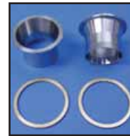
Stainless Steel Taper Valve Kit includes 2 pure stainless extruded sleeves to fit between pipe and exhaust port, to aid in back pressure when drag pipes are used. Kit includes solid copper machined exhaust seals which will not restrict flow. VT No. 30-0312
