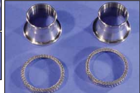
Stainless Steel Taper Valve Exhaust Kit fit into the header at the flange area to compensate for exhaust velocity when large diameter pipes installed. Fits Evo and XL models 1986-up with large O.D. aftermarket pipes. Kit includes 2 valves with gaskets.
