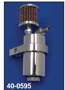
Engine Breather Oil Collector designed to collect the oil mist from breather hose which eliminates engine oil from collecting in air cleaner. Available in polished or chrome plated finish. Features an internal oil baffle that allows the oil and air to separate more efficiently by promoting unrestricted breathing. On top is a high flow air filter that can easily be cleaned. A 90° barbed fitting fits breather hoses perfectly. On the bottom is a drain plug to allow drainage on a regular basis. Measures 5 3/8" x 1 1/2" and includes chrome mounting clamp.
