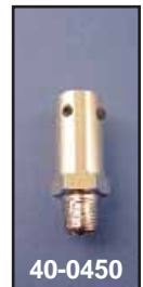
Sifton Breather Canister features enclosed breather filter and tube for attaching to breather cross over lines, which is held in place by set screws. Bottom cover is removable for cleaning.
