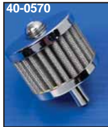
Chrome Crankcase Vent clamps direct to 3/8" breather hose. Unit comes with a 5/16" stud and nut or 1/4" x 20 threaded insert to mount from bracket. Measures 2" diameter x 1 1/2" high. VT No. Type 40-0381 Stud, K&N 40-0570 Threaded
