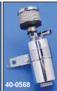
Engine Breather Oil Collector designed to collect the oil mist from breather hose which eliminates engine oil from collecting in air cleaner. Available in polished or chrome plated finish. Features an internal oil baffle that allows the oil and air to separate more efficiently by promoting unrestricted breathing. On top is a high flow air filter that can easily be cleaned. A 90° barbed fitting fits breather hoses perfectly. On the bottom is a drain plug to allow drainage on a regular basis. Measures 5 3/8" x 1 1/2" and includes chrome mounting clamp.
