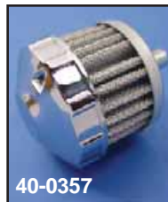
Crankcase Breathers connect to breather hose when stock air cleaner has been replaced. Filters feature chrome tops with washable elements. Bracket can be mounted to transmission case. VT No. 40-0246 includes chrome bracket fastened to body by allen screws, hose fitting is 1/8" NPT threaded into body and can be changed to 90° for special applications.
