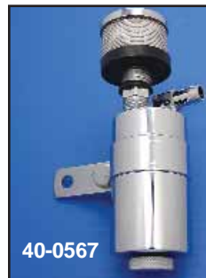
Engine Breather Oil Collector designed to collect the oil mist from breather hose which eliminates engine oil from collecting in air cleaner. Available in polished or chrome plated finish. Features an internal oil baffle that allows the oil and air to separate more efficiently by promoting unrestricted breathing. On top is a high flow air filter that can easily be cleaned. A 90° barbed fitting fits breather hoses perfectly. On the bottom is a drain plug to allow drainage on a regular basis. Measures 5 3/8" x 1 1/2" and includes chrome mounting clamp.
