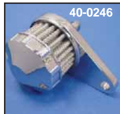
Crankcase Breathers connect to breather hose when stock air cleaner has been replaced. Filters feature chrome tops with washable elements. Bracket can be mounted to transmission case. VT No. 40-0246 includes chrome bracket fastened to body by allen screws, hose fitting is 1/8" NPT threaded into body and can be changed to 90° for special applications.
