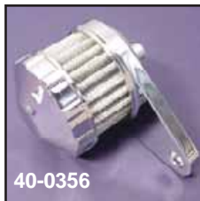
Crankcase Breathers connect to breather hose when stock air cleaner has been replaced. Filters feature chrome tops with washable elements. Bracket can be mounted to transmission case. VT No. 40-0246 includes chrome bracket fastened to body by allen screws, hose fitting is 1/8" NPT threaded into body and can be changed to 90° for special applications.
