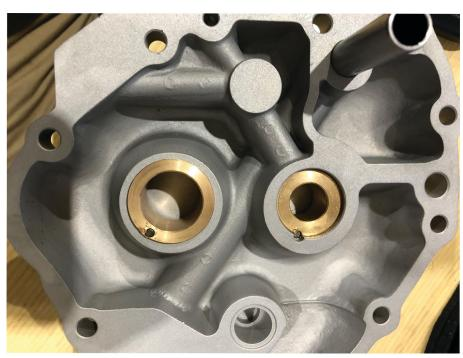
OIL RELIEF HOLES ARE RQUIRED IN BOTH THE PINION AND CAM.
