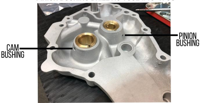
CAM COVER NEEDS TO BE DRILLED DIRECTLY THROUGH THE CAM BUSHING. HOLE FOR PINION MUST BE DRILLED BEHIND/BELOW THE PINION BUSHING.
