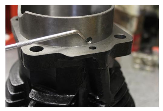
2. Next place cylinder head into case and mark the spot to match the existing hole.
