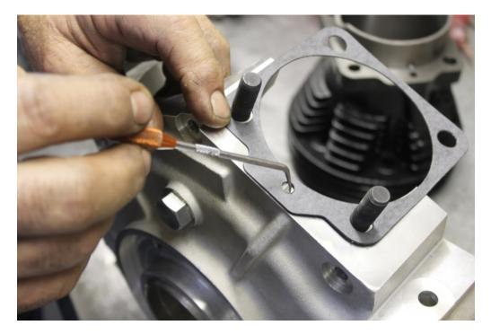
1. First use a gasket to mark locations of holes for drilling in top of the case.
