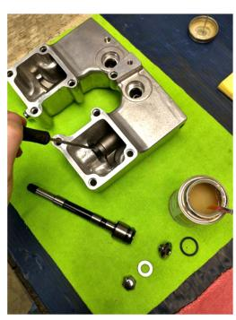
APPLY GASGACINCH VT# 41-0168 TO ROCKER SPACER OPPOSITE SIDE OF ROCKER ARM. \*DO NOT SEAL ARM\*
