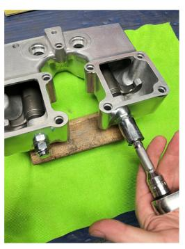
SEAL INSIDE OF HEAD AND ROCKER SHAFT THREADS TO PREVENT WEEPING. INSTALL WASHER AND NUT AND TIGHTEN. THIS WILL HELP ENSURE THE HEADS DO NOT LEAK.
