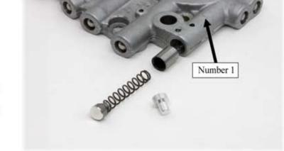
Using a small punch, gently tap out the pin until it no longer retains the spring. (The punch will retain it)
