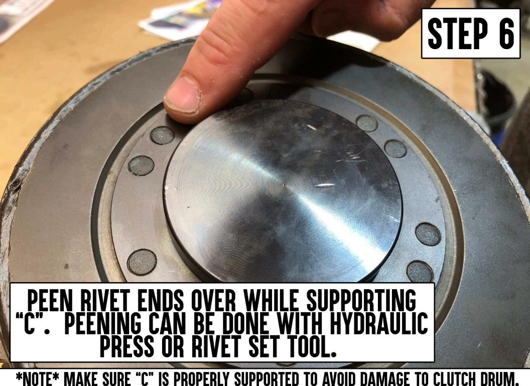
\*NOTE\* MAKE SURE "C" IS PROPERLY SUPPORTED TO AVOID DAMAGE TO CLUTCH DRUM.
