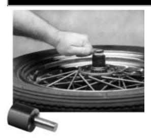
Wheel Bearing Locknut Socket Use on Big Twin and Sportster - 1967-72
