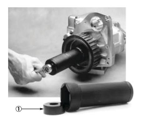
This tool will easily remove and install the left hand threaded nut that holds the trans sprocket on. The pilot is designed to be threaded onto the left-hand thread of the main shaft with the pilot in place. This will stop the tool from slipping when torquing 100 to 120 ft lbs. Apply lube to threads of tool.
