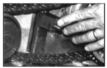
2. Remove the factory chain tensioner, but DO NOT remove the inner slotted adjustment bracket that is held in place with two flush screws. Then slip the GUIDE PLATE (with the large steel block on the end) over the carriage bolt and slide it back against the factory slotted adjustment bracket with the block facing you. In some cases, the length of the guide plate may need to be shortened to fit your primary case. This can be accomplished by grinding the end as required.
