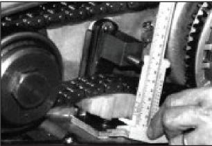
5. Place the other GUIDE PLATE with the bevel-cut edges facing inwards (towards the SHOE). Keeping the M6 held at a 90° (right angle) to the lower primary chain, torque the nut to 33 ft. pounds
