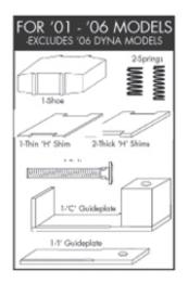
4. Place the thin 'H' shim under the springs and measure for 5/8" from bottom of the SHOE to the to of the SHIM. If you need more than 3 SHIMS this may indicate that your primary chain is worn and should be replaced.
