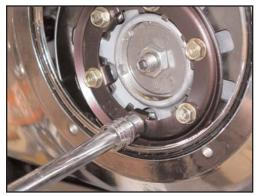
1. Remove the derby cover and stock spring plate. Break loose all six screws on the spring plate and back them out evenly Once they are clear of the spring plate, they can be removed with your fingers.
