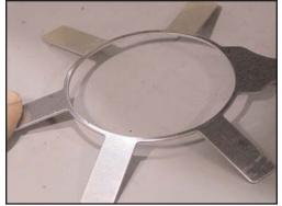
3. The spider that comes with the kit as a flat piece of steel needs to have its fingers or tangs bent a little to conform with the curve of the stock diaphragm spring.
