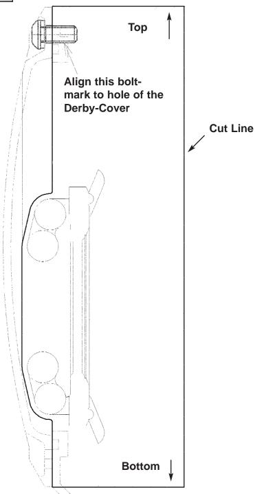
To check the clearance between the VPC and Derby Cover. Cut the "Template" and Follow along the Cut Line
