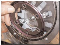
2. The spring plate is now free to be removed from the clutch. **NOTE: If replacing the diaphragm clutch it will be necessary to remove the primary cover. Refer to the service manual on primary cover removal.**
