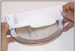
**WARNING:** Use the template and provided instructions to check for proper clearance.
