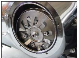
4. Place the spider inside the clutch spring with the fingers pointing out as shown. The spider can be manipulated through the slots in the diaphragm spring without removal.
