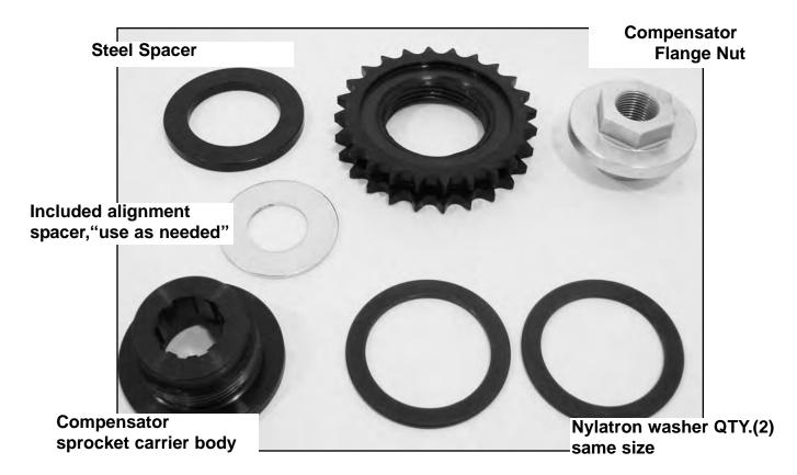
On Softail models 1986-1999 the removal of the stock .200" compensator spacer and use of the .125" spacer supplied in kit, may be needed to achieve correct primary chain alignment.
