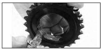
5. Evenly apply a small amount of Anti-Sieze to all of the threads of the compensator sprocket.
