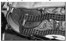
3. Remove existing sprocket or compensator & spacer. Refer to Harley manual for removal instructions for your year and model bike..
