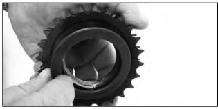
6. Lightly grease and install (1) of the Nylatron washers into one of the recessed pockets of the compensator sprocket. "Either side is OK"
