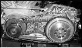
2. Drain primary fluid, and remove outer primary cover and gasket.
