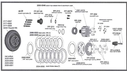
2050-0050 .... CLUTCH HUB / COMPLETE ASSEMBLY/FITS 1990 & UP BIG TWIN 2050-0049 .... CLUTCH HUB w/STEEL INNER & ALUMINUM OUTER ONLY PP-201-90 .... CLUTCH HUB / STEEL INNER / FOR EVO SPLINED SHAFT
