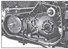
Install the sealed bearing (PP-216)
