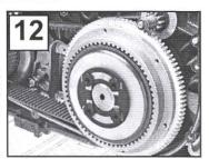
Bend the locking tabs over as shown! Belt should have 1/2"- 3/4" of up & down play when the drive train is cold. Re-install the outer primary cover and check belt clearance. Install a louvered or vented derby or inspection cover, and you're ready to ride. Check belt tension after the drive train reaches normal operating temperature (15-20 minutes of riding at 55 MPH in ambient air temperature of 68 degrees). The belt should feel snug but not excessively tight!
