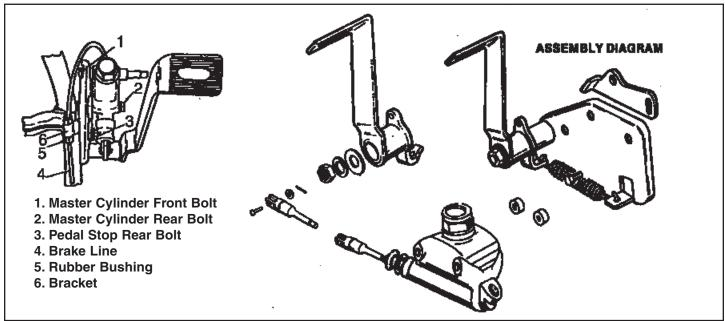
1970-up FL-FX-FXR Control includes either chrome or plain cast iron master cylinder. Complete bolt on forward control for these years. Unit with unchromed master cylinder includes chrome cover for cylinder.
