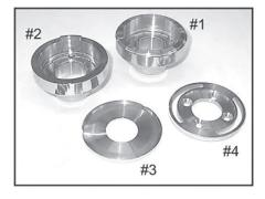
1. See Fig. 1: Drill 4 holes in the lower Triple Tree using the Fork Stop Ring (#4) s a template.
