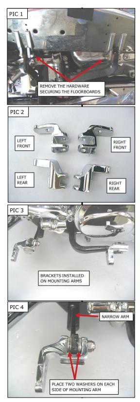
3.Refer to PIC 2 to determine the left (sitting on the bike) brackets and install the left brackets on the mounting arms on the bike. PIC 3; secure the arms with the 1/4"-20 x 1-1/4" shoulder bolts and 1/4"-20 nylon locking nuts from the hardware kit.
