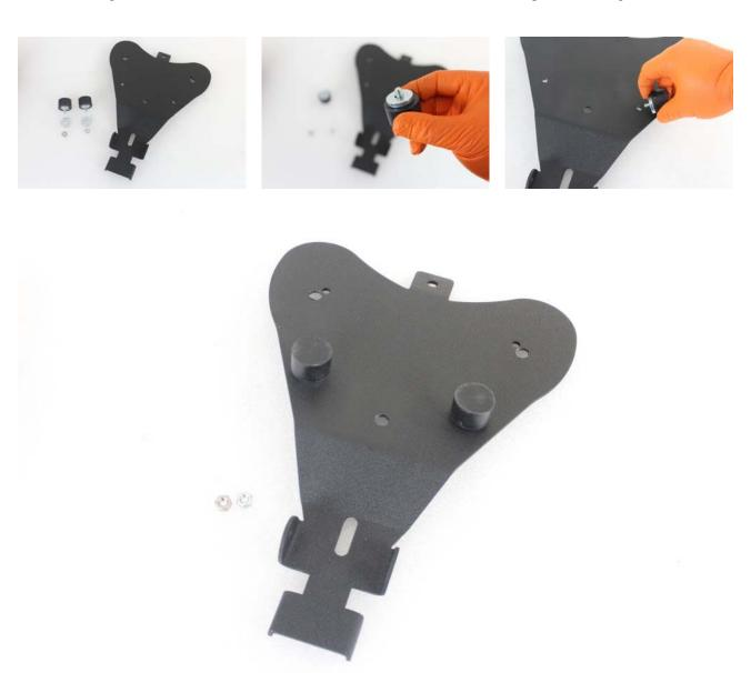
Now it's time to attach your seat plate directly to your seat. Flip your seat upside down and line the holes up with the bolts in your seat. Finally place washers and nuts on bolts and tighten.
