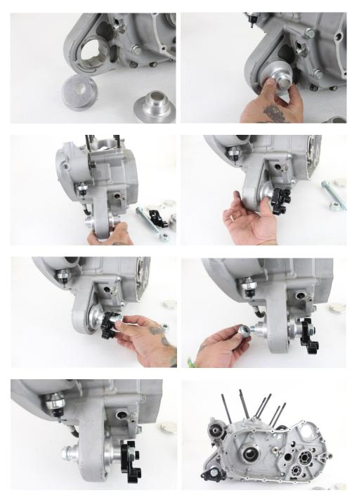
**Step 3** – Attach rear mounts as demonstrated below. Please note rear motor mount covers are only used for hardtail installations. The covers cannot be used on softail installations.
