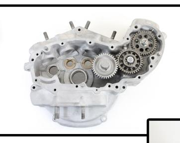
IDLER INSTALLED WITH GEARS 10-1299 & 32-1256
