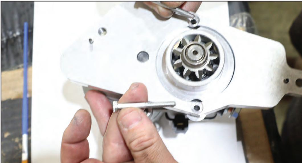
Install Plate Provided Mount Screw VT No. 500-229
