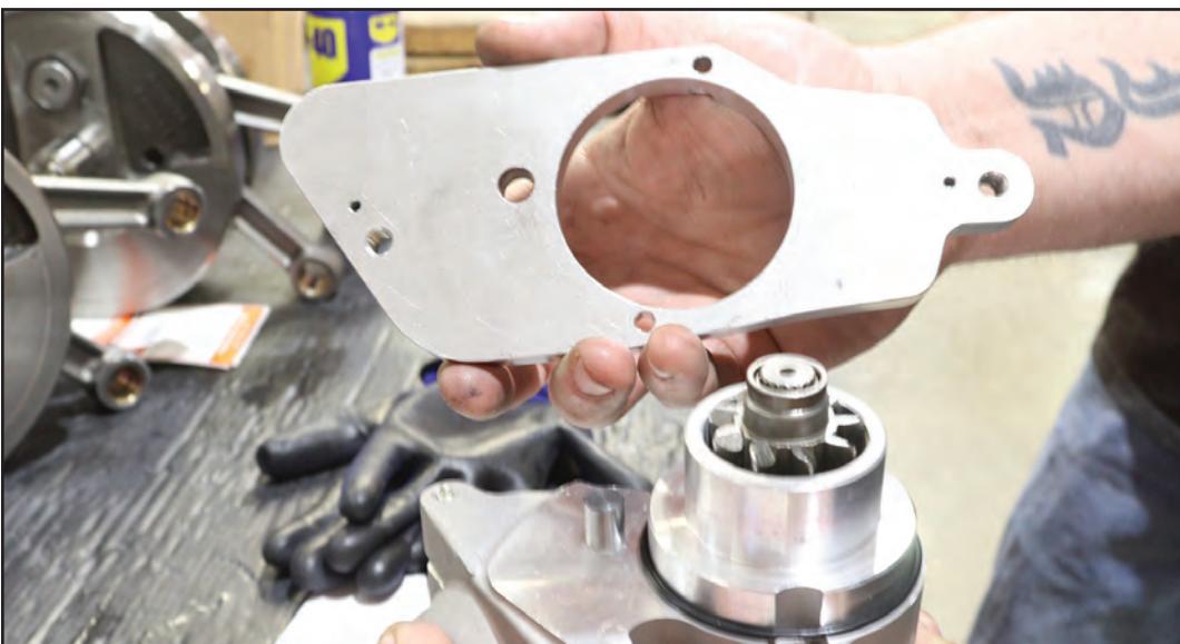
Install Plate to Starter
