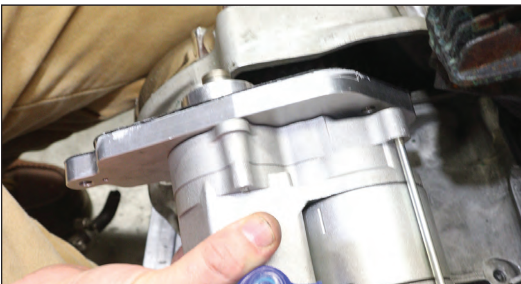
Install Unit, Lining up mount pins.
