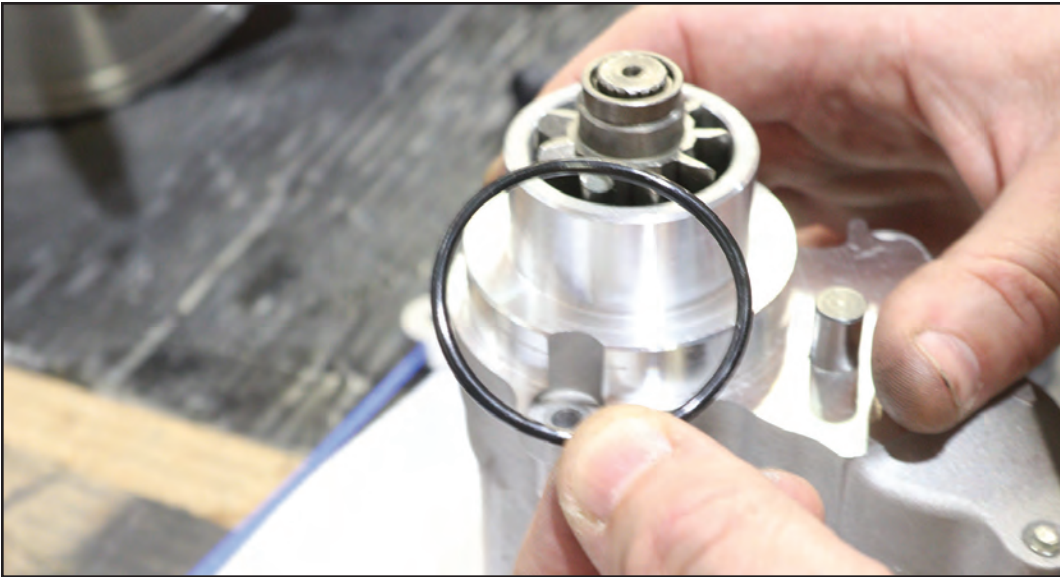
Install 1-2 O-Ring Provided VT No. 14-0537
