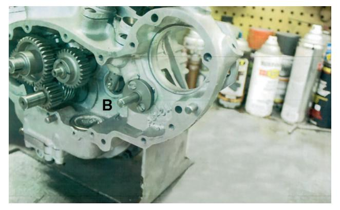
NOTES FOR PHOTOS: Modification to the right side engine case point "B", must be welded to build platform for the new stud location. Also point "A" on cam cover must be welded up and relocated. A WR cam cover is available, VT #10-1947 WR 45" Cam Cover Alloy. Magneto assembly should be screwed in place by 5/16" screws. Original right engine case and generator holes in cam cover must be enlarged to 5/16".
