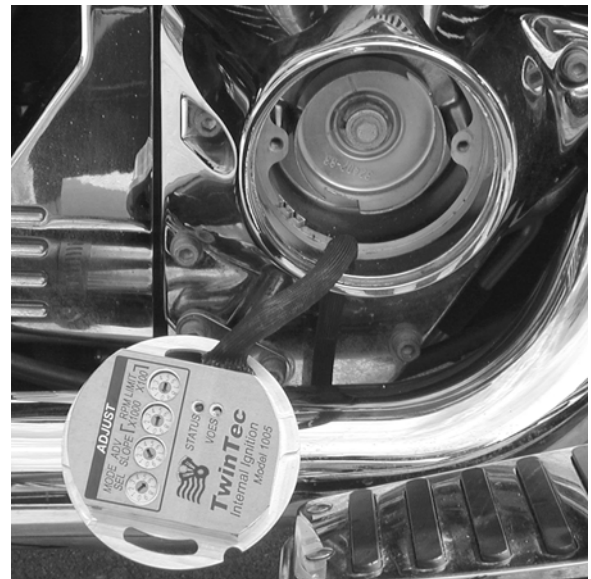
Figure 1 - Feeding Harness Thru Exit Hole
