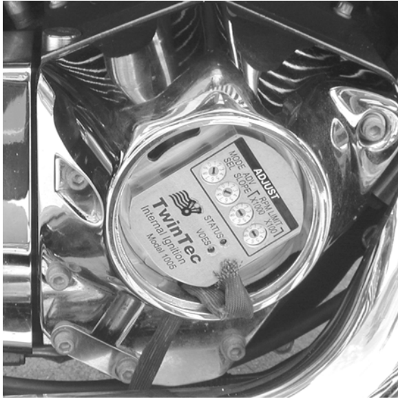
Figure 2 - Installing Unit (Note Orientation)
