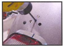
2. Position the rubber gasket over the 3 OEM mounting holes. Mark and drill a hole for the wires. Place a small rubber grommet in hole to prevent chaffing of the wires.
