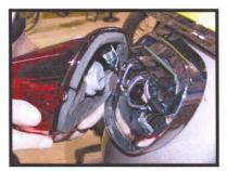
8. Reinstall the OEM taillight lens.
