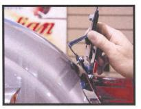
1. First remove the OEM license plate bracket. See service manual if needed.
