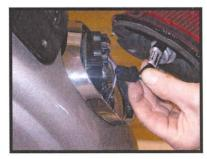
4. Remove the OEM taillight lens and unplug the assembly from the bike.
