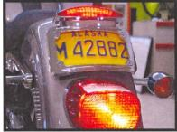
9. Reinstall the OEM taillight lens.
