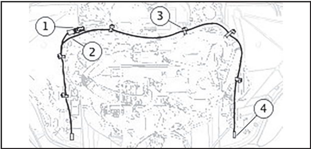
1 Accessory connector {299} 2 Jumper harness 3 Cable Strap (6) 4 Edge Light Connector (2) Figure 4. Fairing Edge Lights, Harness Connection
