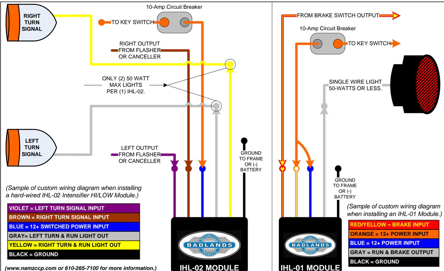
The wire colors in the drawing are used for reference only based on the colors we use on our module. When installing either the IHL-01 or IHL-02 3 HI/LOW Intensifier Modules on a factory model, be sure to consult your bikes service manual for exact wiring diagrams and color descriptions to achieve proper installation.
